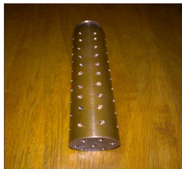
Fig. 4: Porous copper rod for extended heating.
